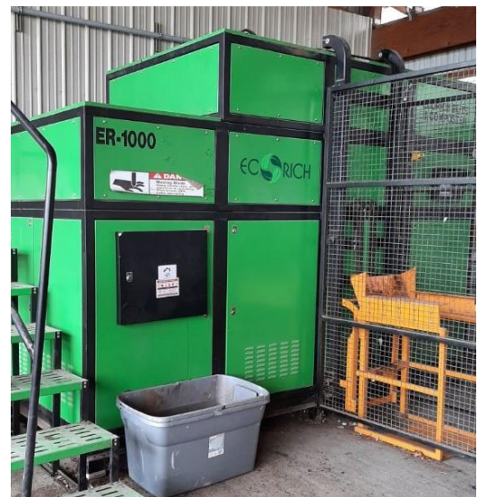
Figure 3 - EcoRich Food Scrap Composter at the Greenport Solid Waste Station Photo by @ClimateSmartClaverack
